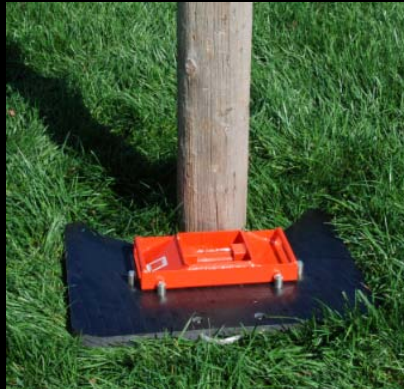
Base plate & pole puller pad positioned within the bushings
